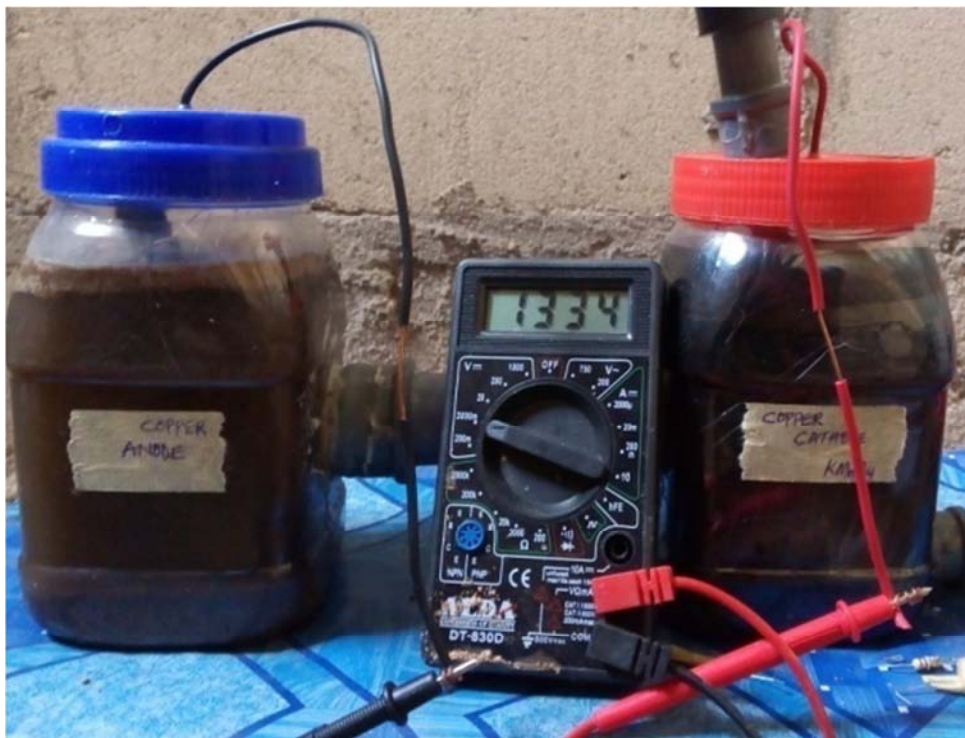
Figure 1. Dual chamber MFC showing voltage generated on multimeter (DT-830D Series).
