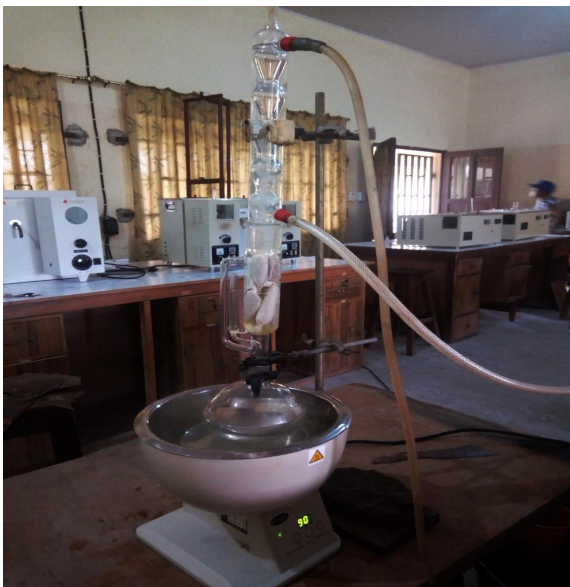
Plate 3.1: Soxhlet Extractor set up in the laboratory
