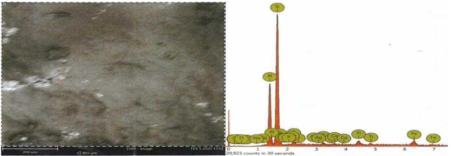
Figure 4.1. SEM-EDS result of clay sample A
