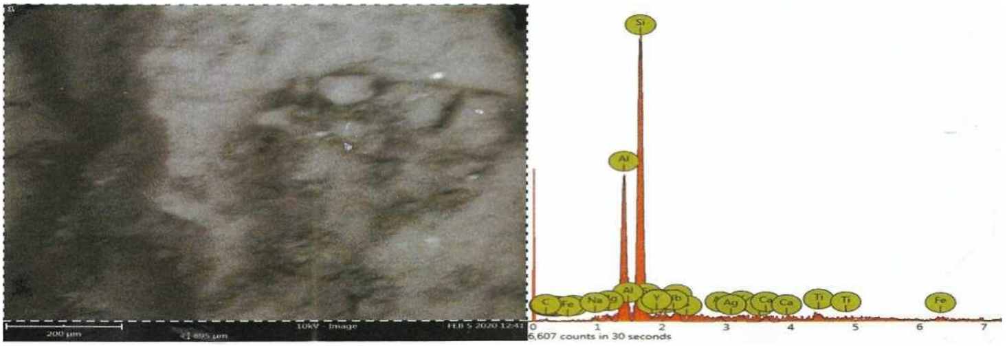
Figure 4.4.SEM-EDS result of clay sample D
