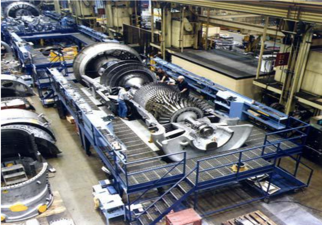
Figure 2.4: GE Frame 7F turbine during manufacture on a test bed in an OEM facility showing rotor in half the casing (Source: GE Power Systems).
