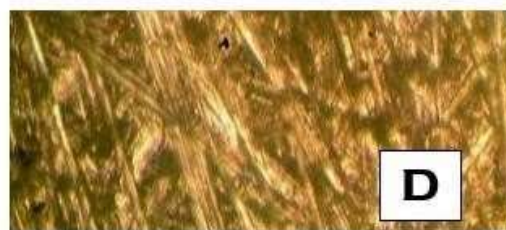
APPENDIX B1: Micrographs (X 200) of mild steel coupons: (A) before immersion, (B) after immersion for 24 hours, (C) after immersion for 72hours, and (D) after immersion for 120 hours.
