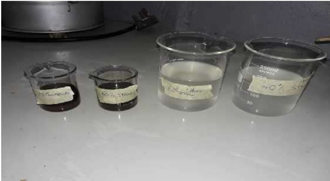
Figure 3.6: The Emulsified oil-water separated
