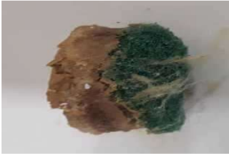
Figure D: Fouled Membrane
