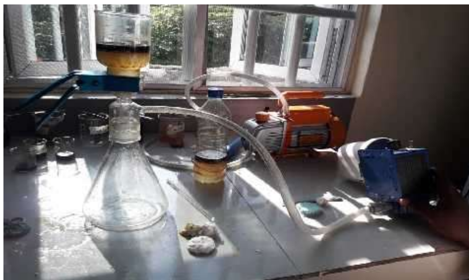
Figure 3.5: Membrane Separation Process using vacuum pump
