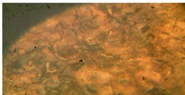
Plate 1: Micrograph of sample ductile iron (control)
