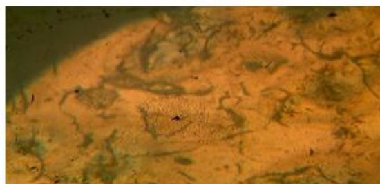
Plate 4: Micrograph of sample austempered at 420°C
