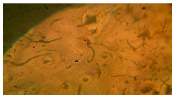
Plate 2: Micrograph of sample austempered at 240°C
