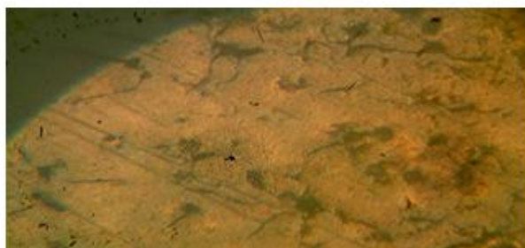
Plate 3: Micrograph of sample austempered at 350°C
