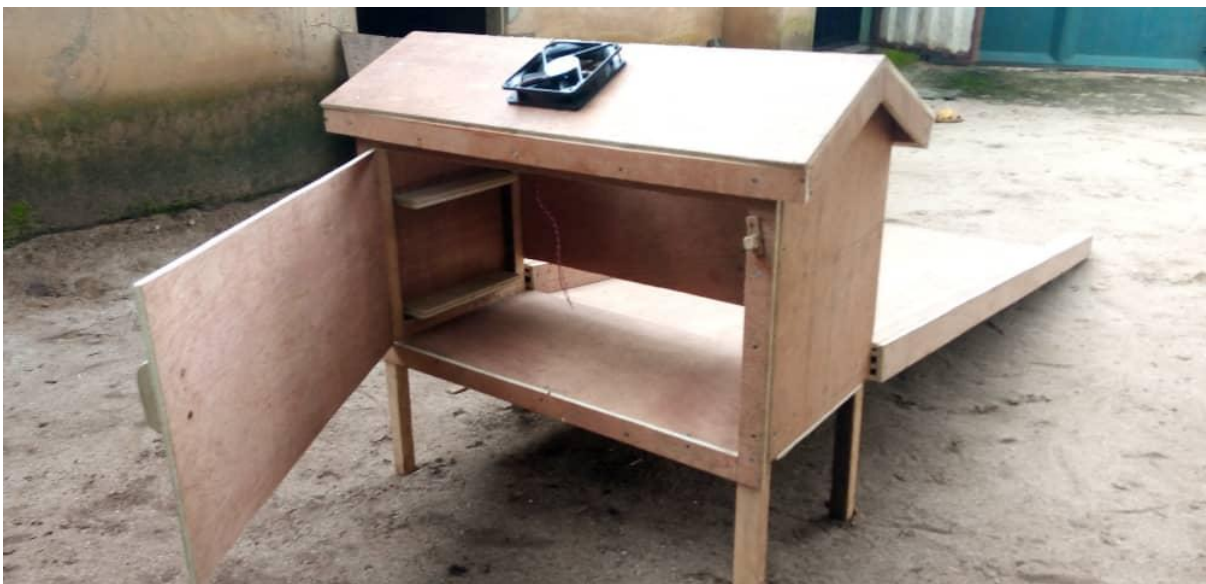
Plate A6: Location of air entrance into the drying chamber
