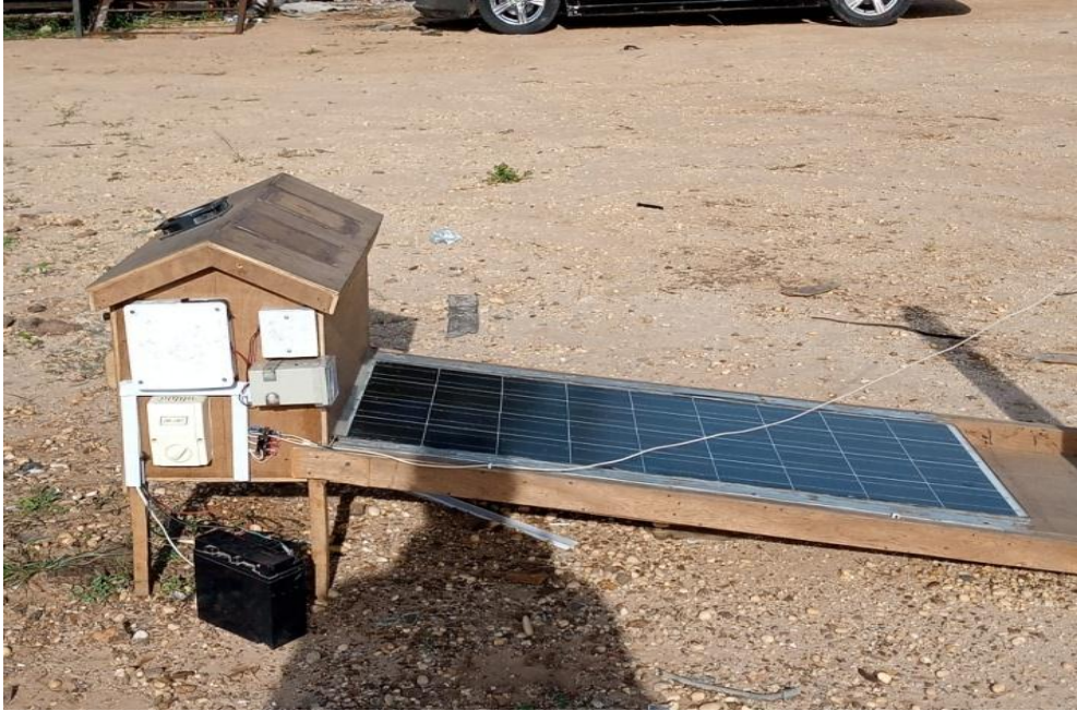
Plate A1: Side view of the PVT powered solar dryer at the test location
