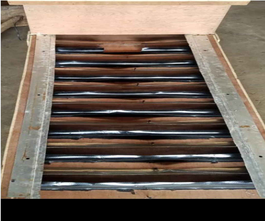
Plate A5: Configuration of the flow channel before installing the PV panel
