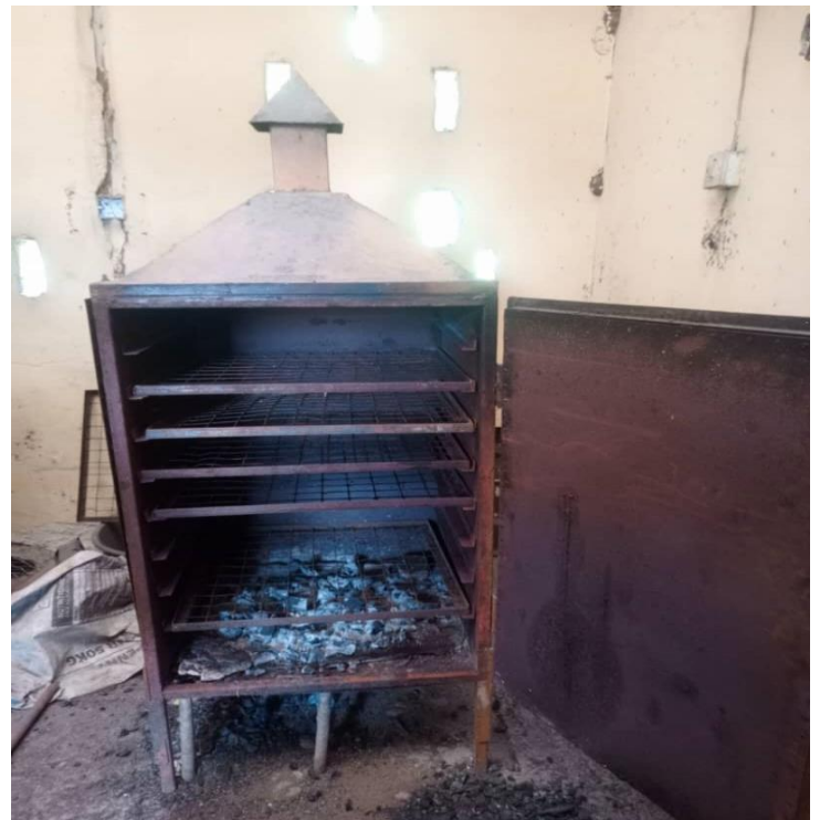
Fig 5: Diagram of Altona-type smoking kiln
