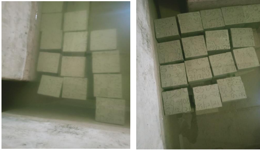
Plate 3.12: Curing of cement-metakaolin blended concrete cubes
