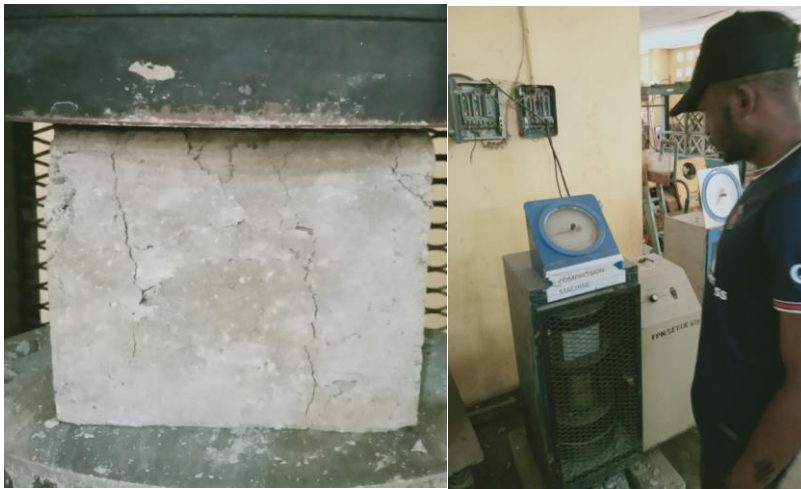
Plate 3.13: Compressive strength testing of cube samples
