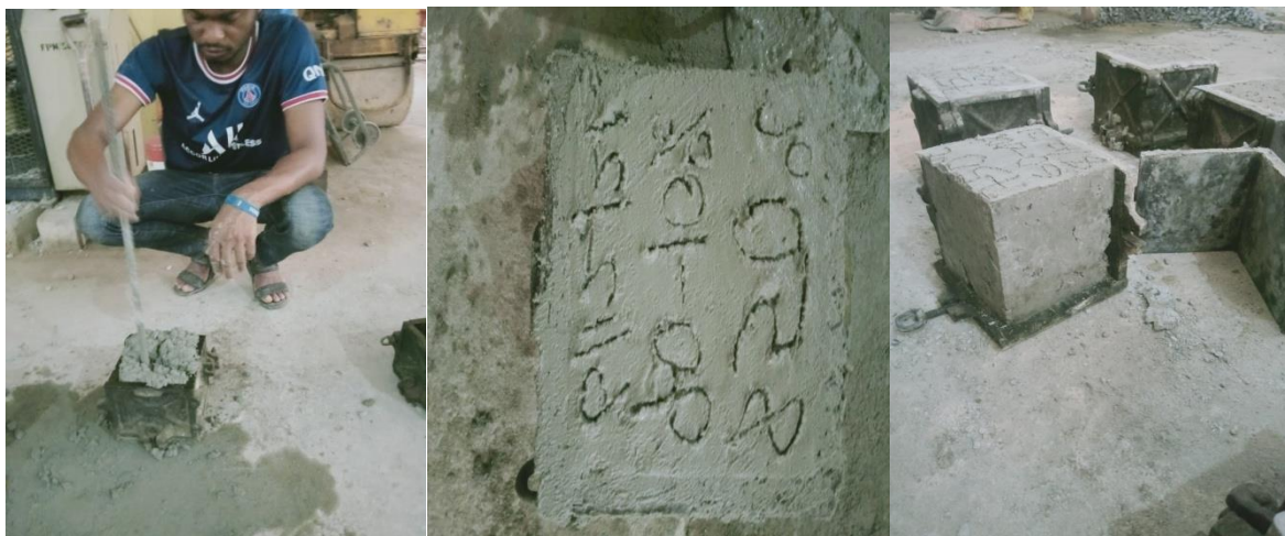
Plate 3.11: Moulding and de-moulding of cement-metakaolin blended concrete cubes
