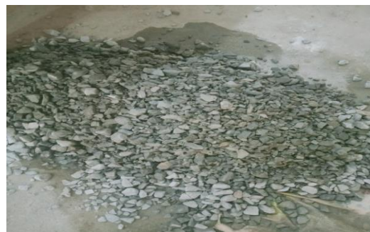
Plate 3.6: Sample of granite chipping
