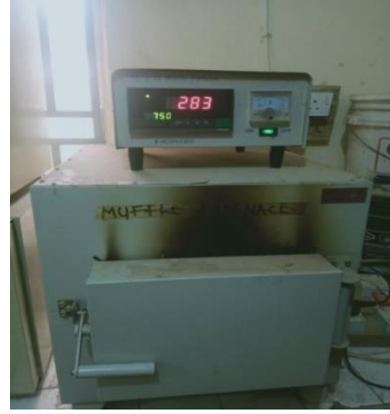
Plate 3.2: Calcinations of kaolin
