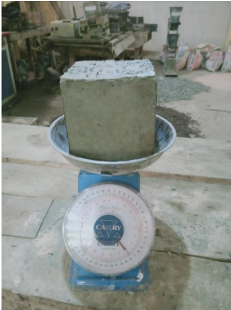
Plate 3.14: Cement-metakaolin blended concrete cubes for water absorption test
