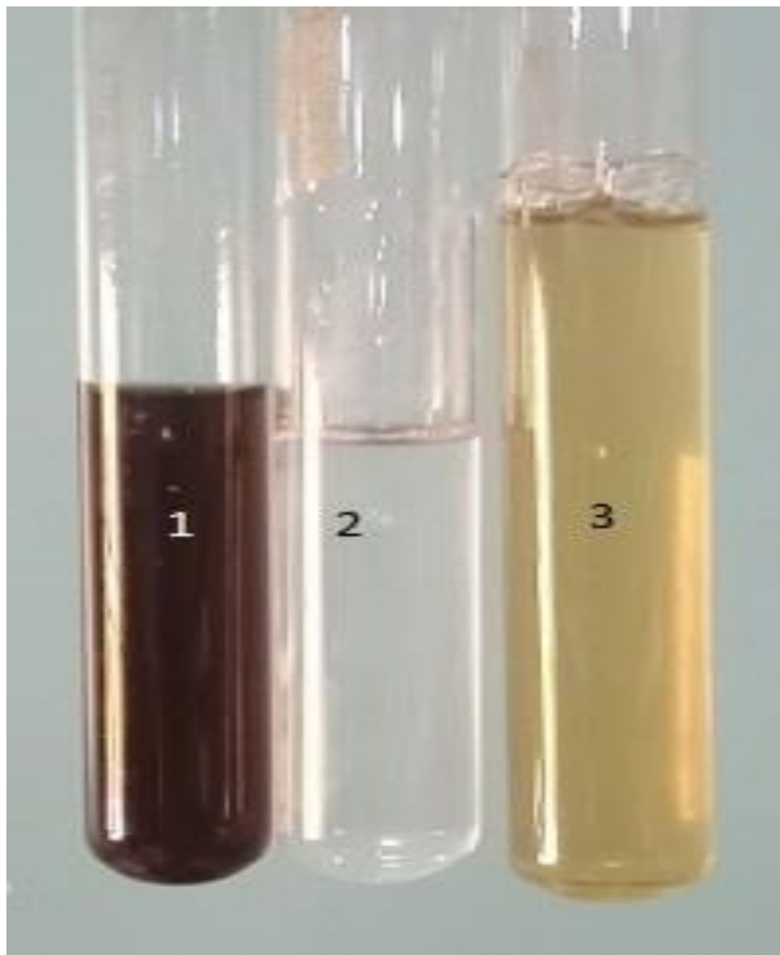
Figure 4.4: Colour change during silver nanoparticle synthesis showing colour of the extract (1), colour of the silver nitrate solution (2), and colour of reaction mixture upon addition of the extract to the silver nitrate solution (3).
