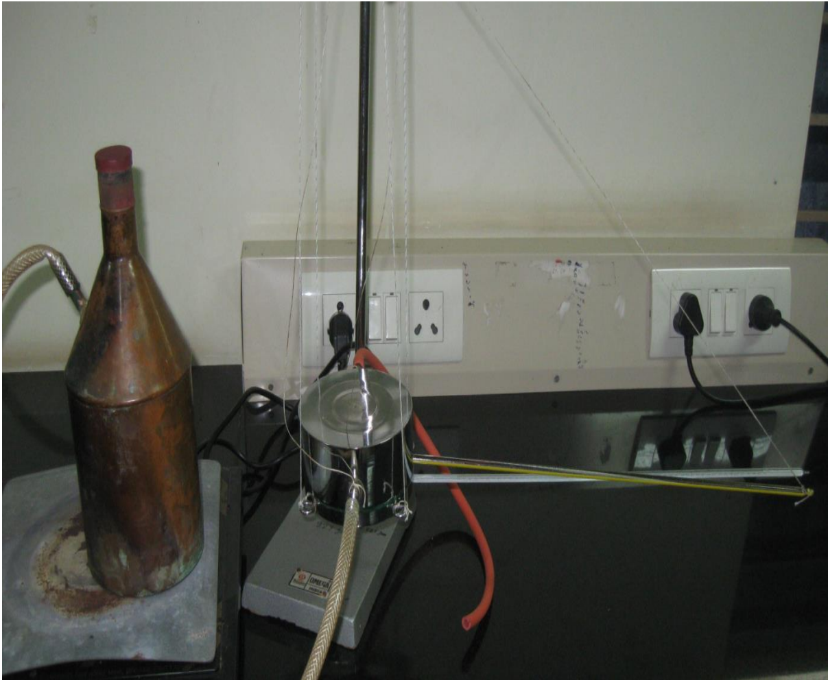
Plate 3.5: Photograph of Thermal conductivity measurement setup
