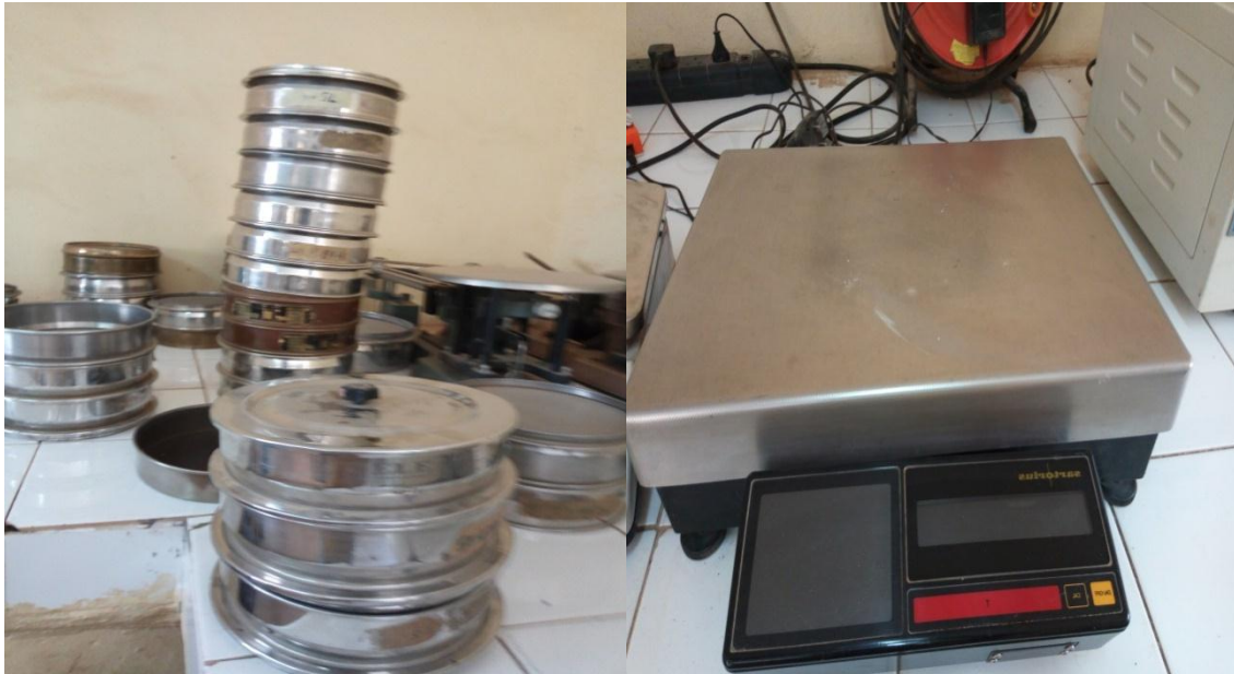
Figure 3.4: Diagram of sieving equipment and digital weighing machine
