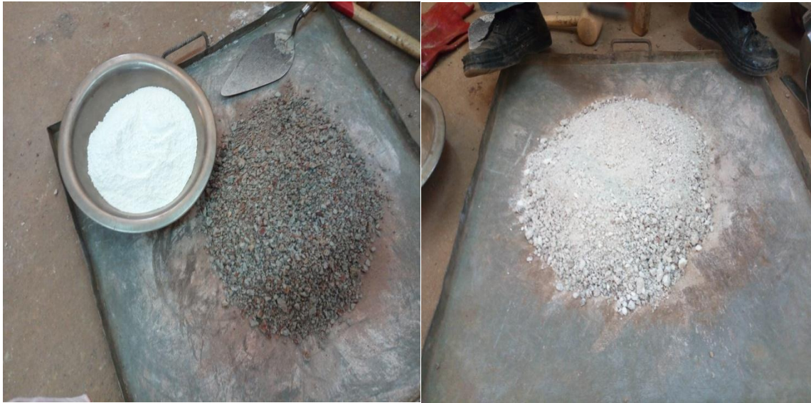
Figure 3.9: Representative expansive soil sample mixed with hydrated lime set for stabilization
