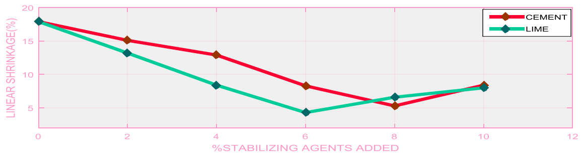
Figure 4.3.7: Variation of linear shrinkage (LS) of expansive soil derived from Imo Shale Formation with different percentages of cement and lime
