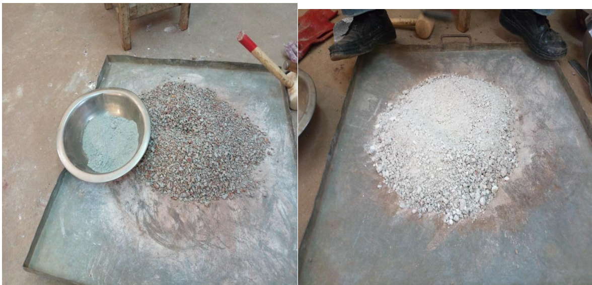
Figure 3.10: Representative expansive soil sample mixed with Dangote cement set for stabilization
