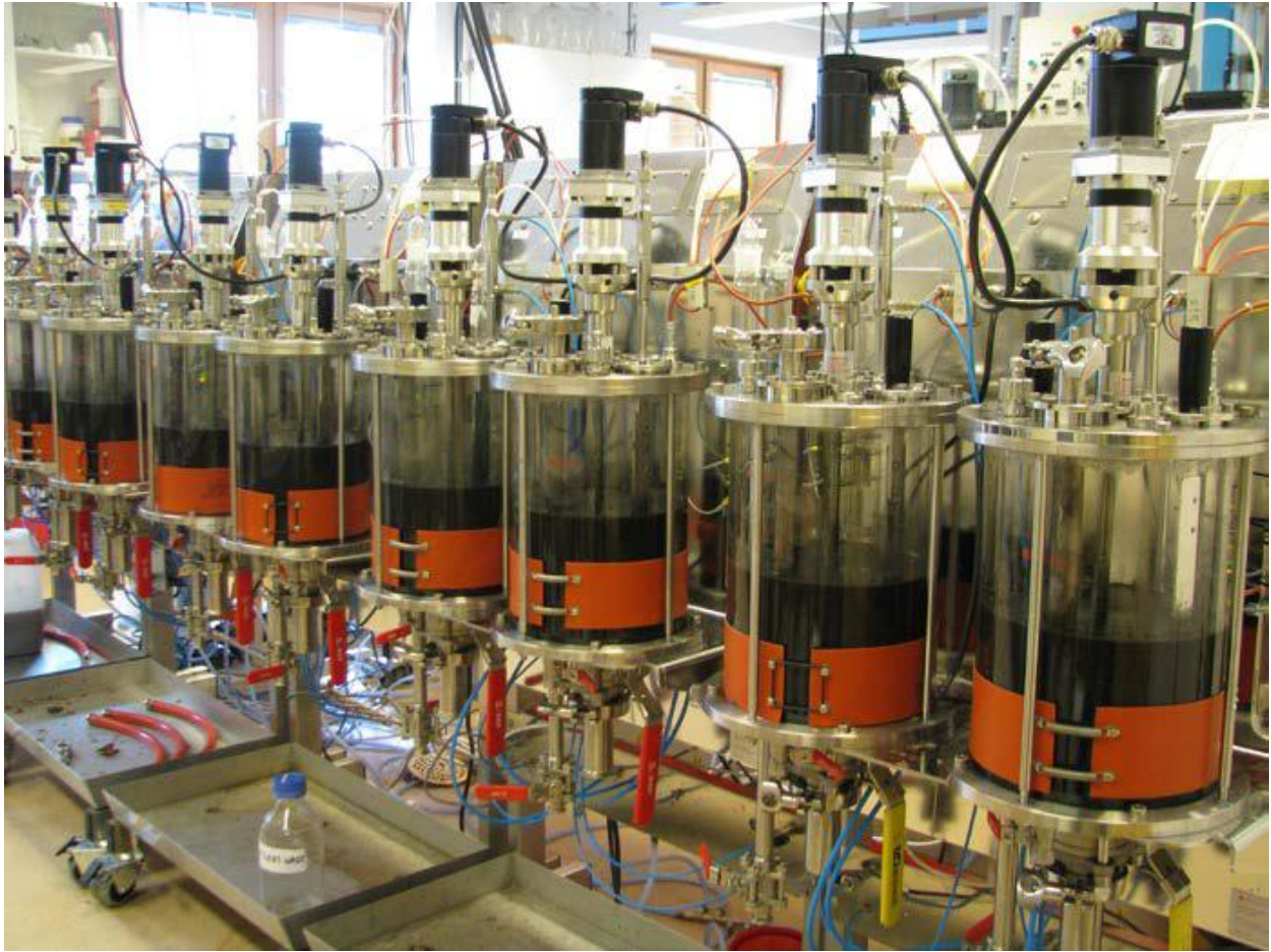
Figure 2.5: Laboratory-scale semi-continuous stirred tank reactor (CSTR) (Sun, 2015)
