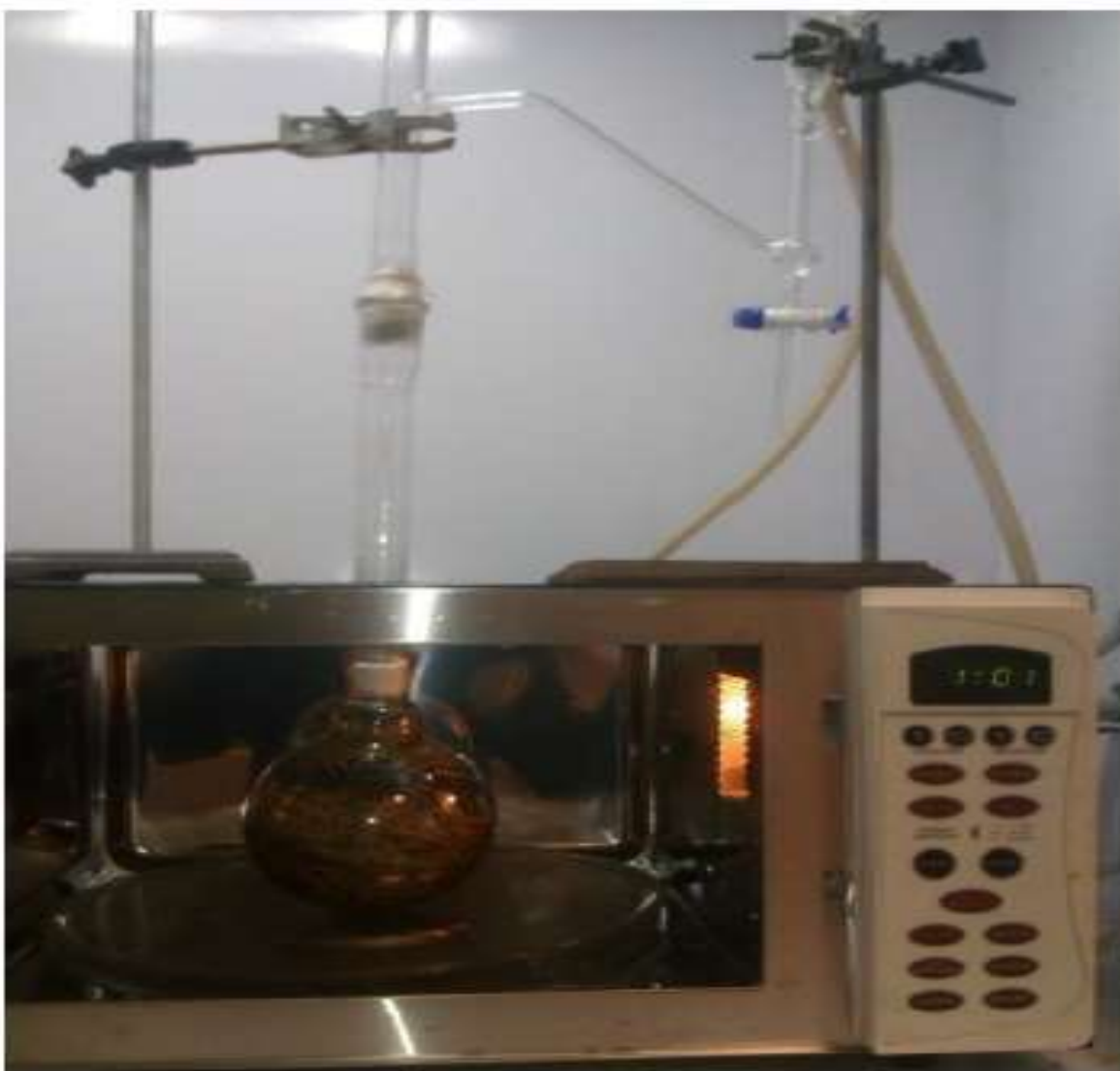
Figure 3.3.A Microwave assisted extraction set-up (containing, retort stands, condensers, and flat-bottomed flask holding the samples under extraction).
