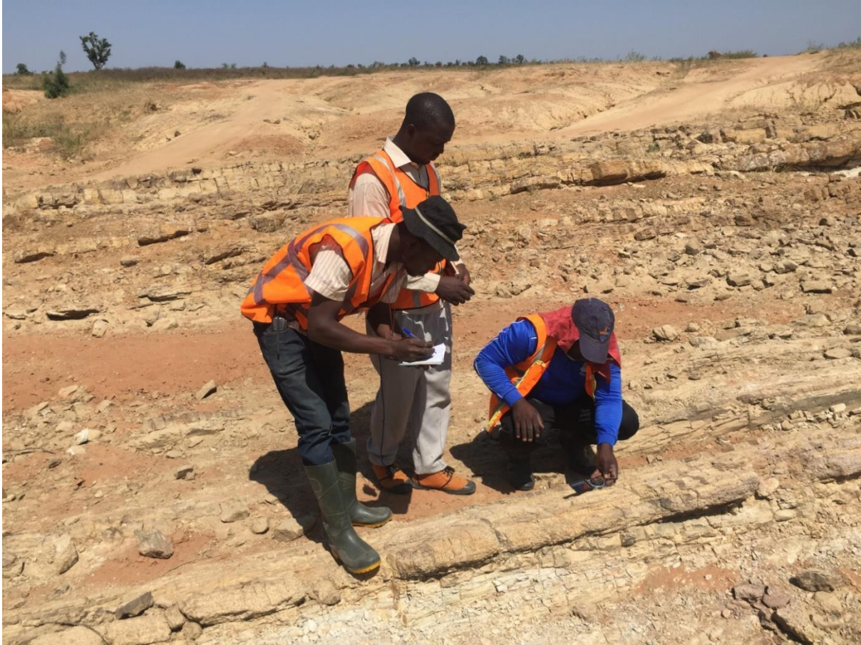
Apendix i: Measuring the dip and strike of an exposed outcrop (Limestone) in profile 2 zone 2
