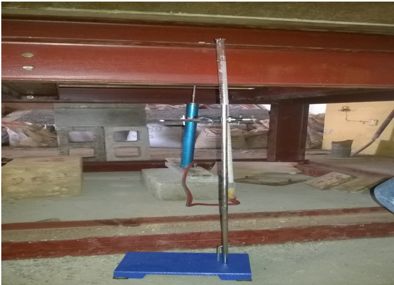
Plate 3.2: Deflection measurement using principle of incompressibility of water
