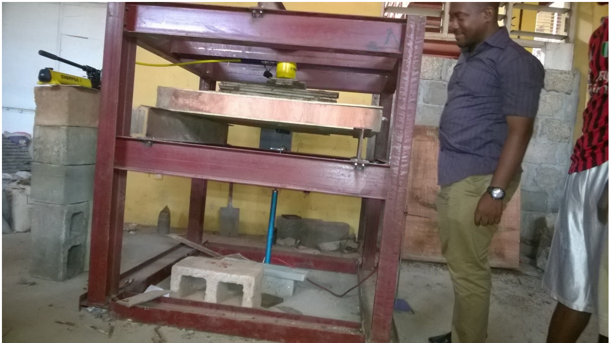
Plate 3.1: Arrangement of slab during crushing as required by BS EN 12390-5:2009
