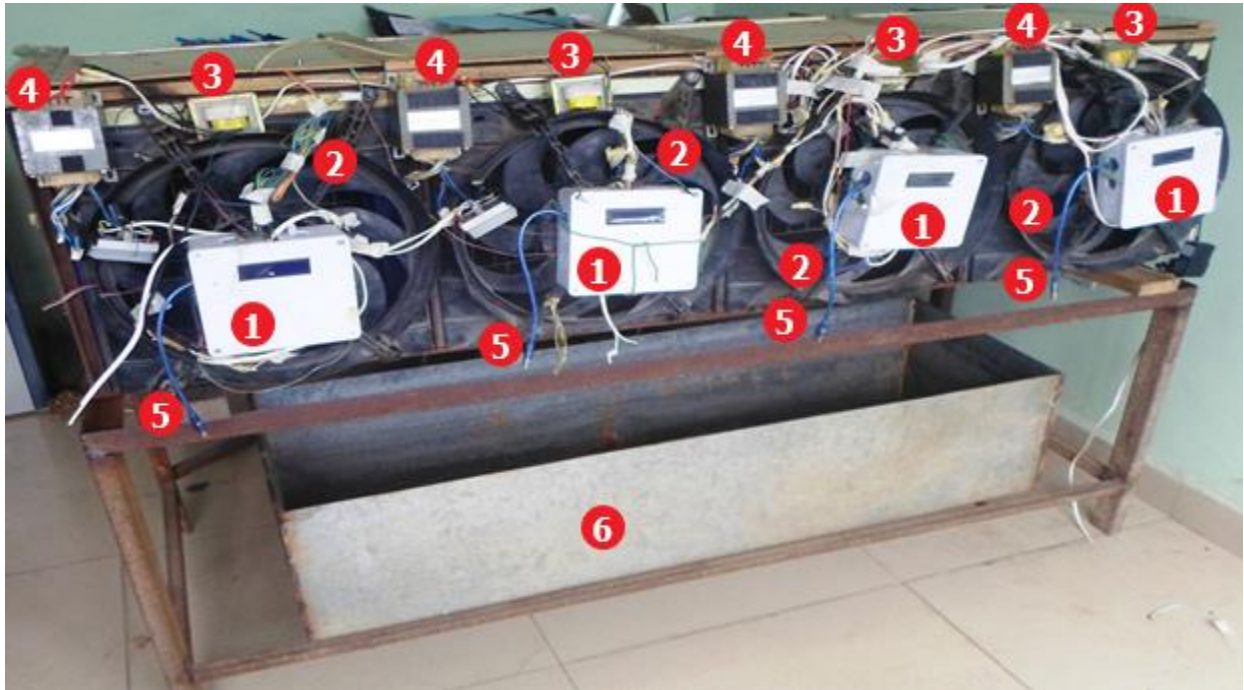
Plate 3.1: Front view picture of evaporative test rig. (1. Data acquisition/control and display box; 2. Suction fan; 3. Pump transformer; 4. Fan transformer; 5. USB Cable; 6. Water sump)
