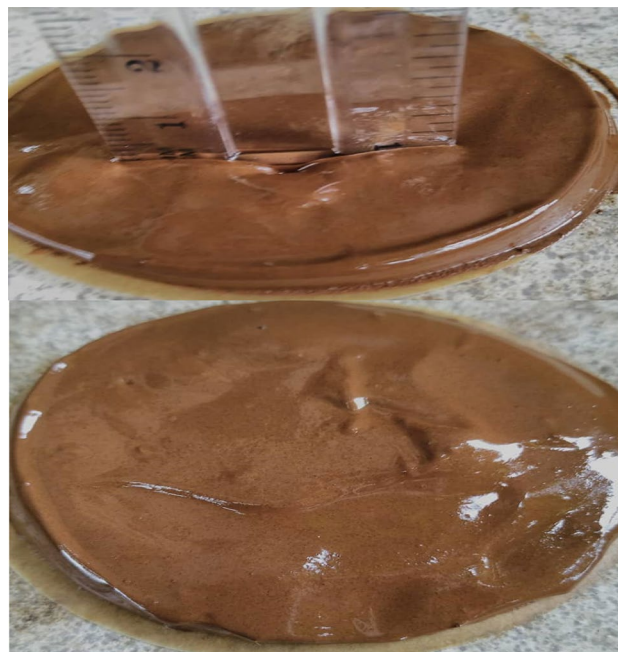
Fig. 9 Filter cake from the filtration test and its measurement
