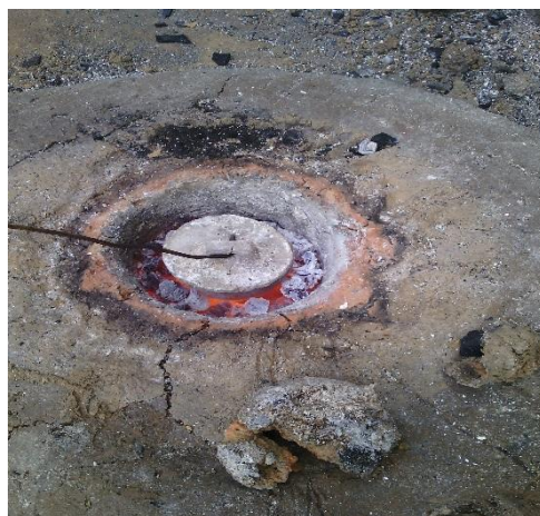
Plate 3.4 firing in progress of the glass in a ceramic crucible with lid.
