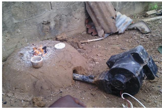
Plate 3.3 monolithic charcoal furnace firing the glass batch with air supply by a DC powered electronic blower constructed for this work.
