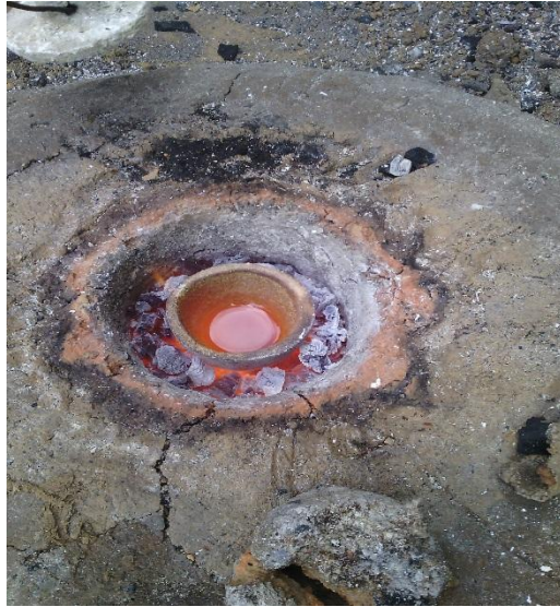
Plate 3.5 after about 2hour of firing crucible is opened showing molten glass.
