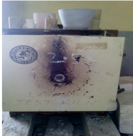
Plate 3.11 electric test kiln used for annealing
