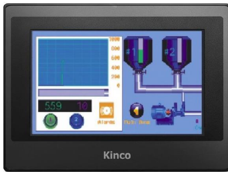
Plate 2.12: Screen Touch HMI (OFF/ON) with trends (Lagari, Nasiakou, Fainti, Mao, Tsoukalas, Bean, & Alamaniotis, 2016)
