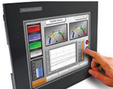
Plate 2.8: Metering device on the HMI Operators panel (Gupta et al, 2018).
