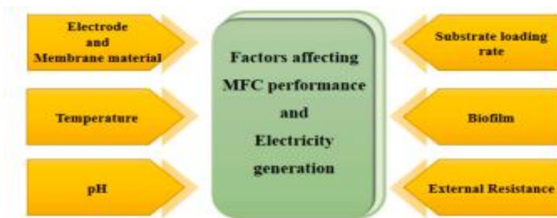
Figure 2.2: Flowchart of parameters depicting MFC performance for bioelectricity generation. Source: Nawaz et al., (2022)
