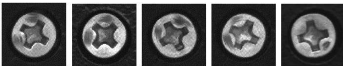
Figure 3.7: Surface dirty screws.
