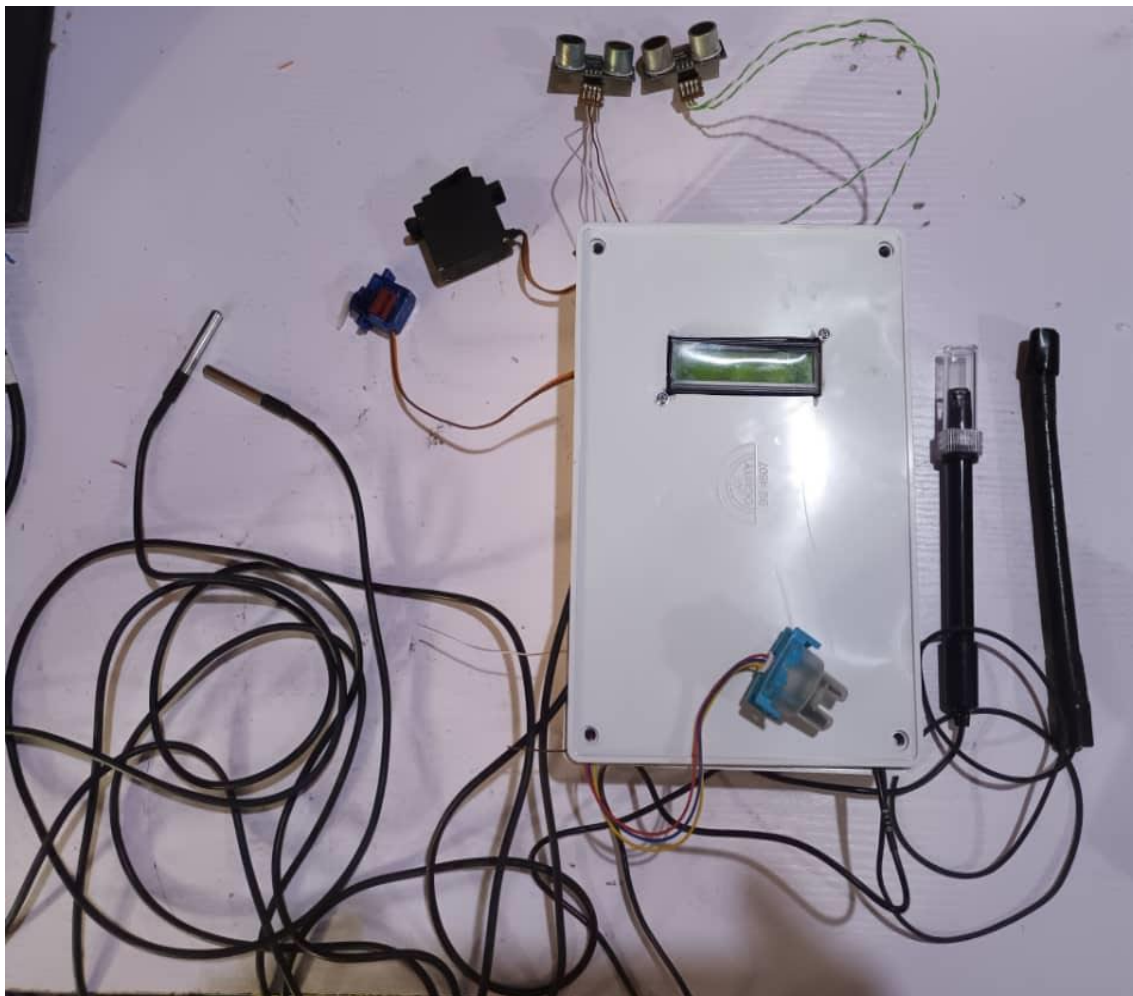
Plate 3.19: Snapshot of components and casing containing circuit of implemented smart electronic system for optimum water quality maintenance in warmwater fish culture
