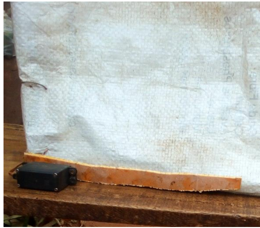
Plate 3.18: Snapshot of installed servo motor-based windbreak
