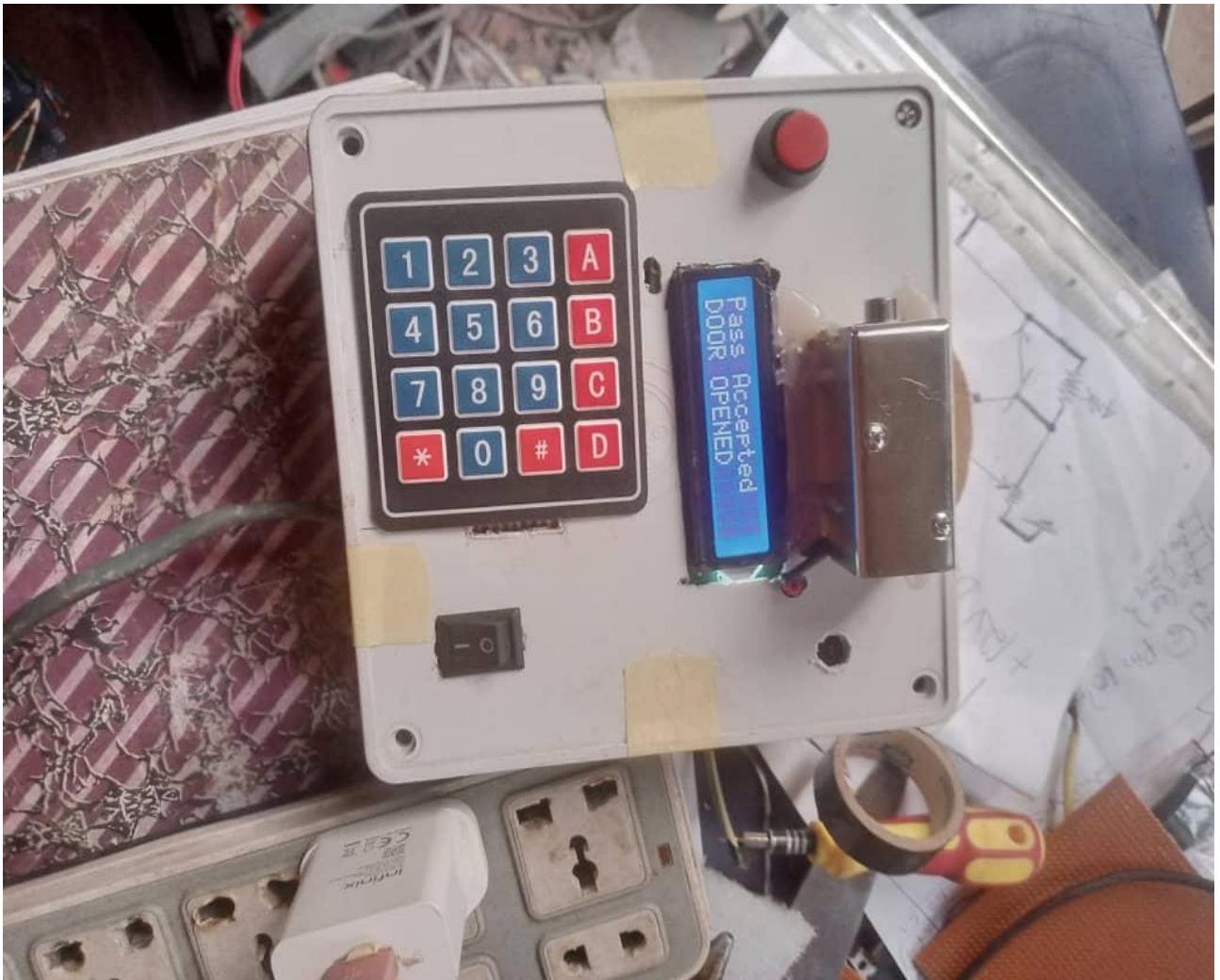
Plate 4.3: The smart door lock in operation showing access granted
