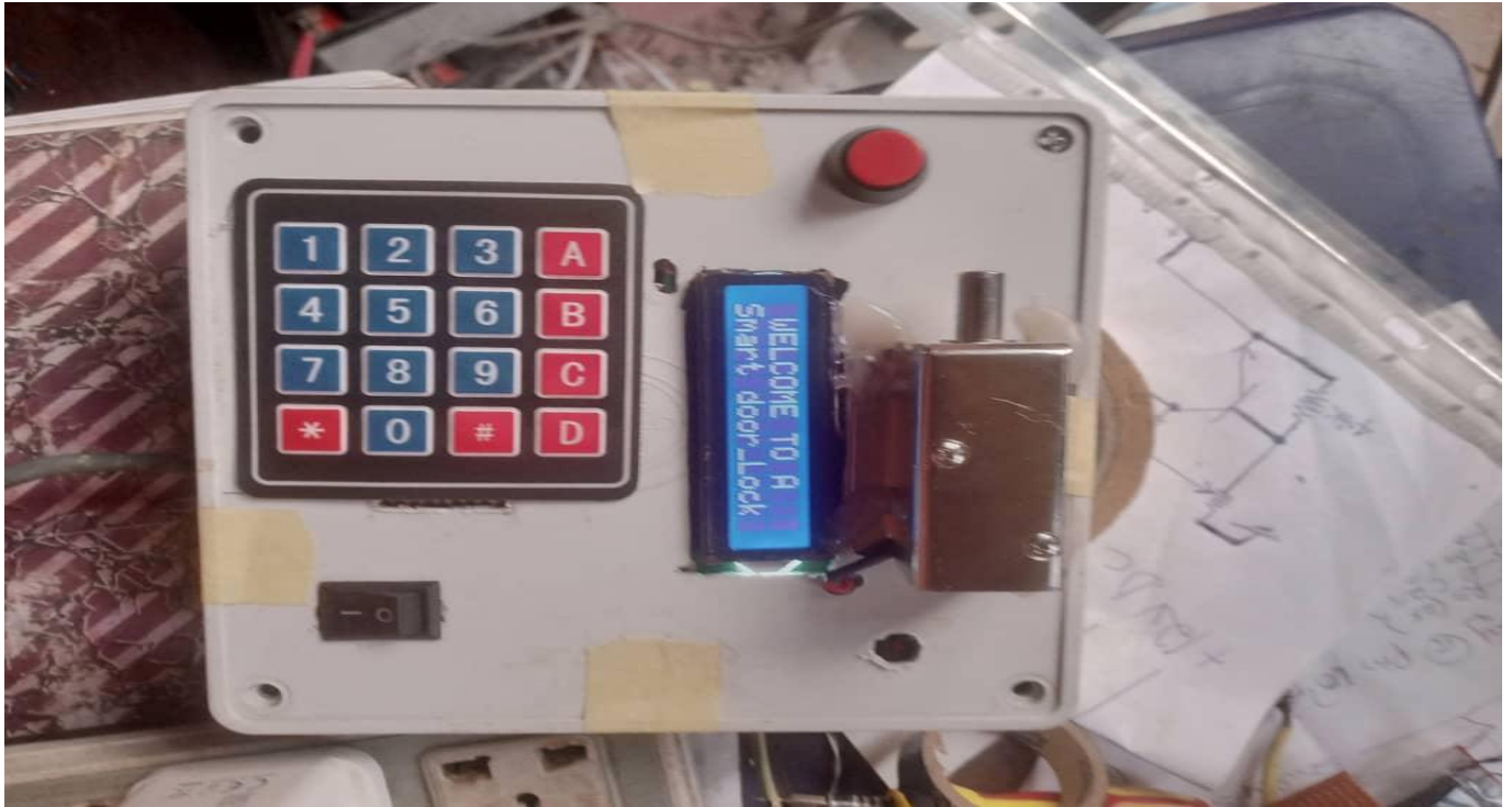
Plate 4.2: A Smart door lock system showing power up state
