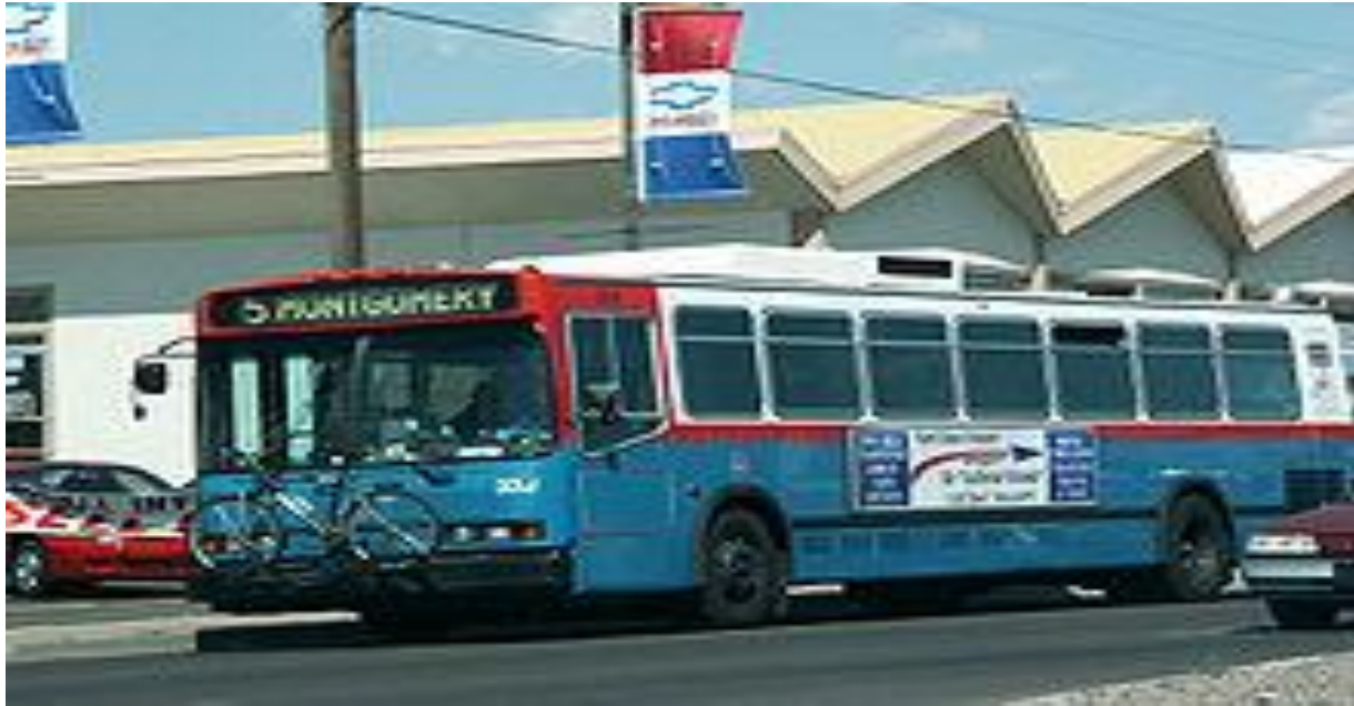
Fig 2.2: A CNG powered high-floor Neoplan AN440A, operated by ABQ RIDE in Albuquerque, New Mexico.
