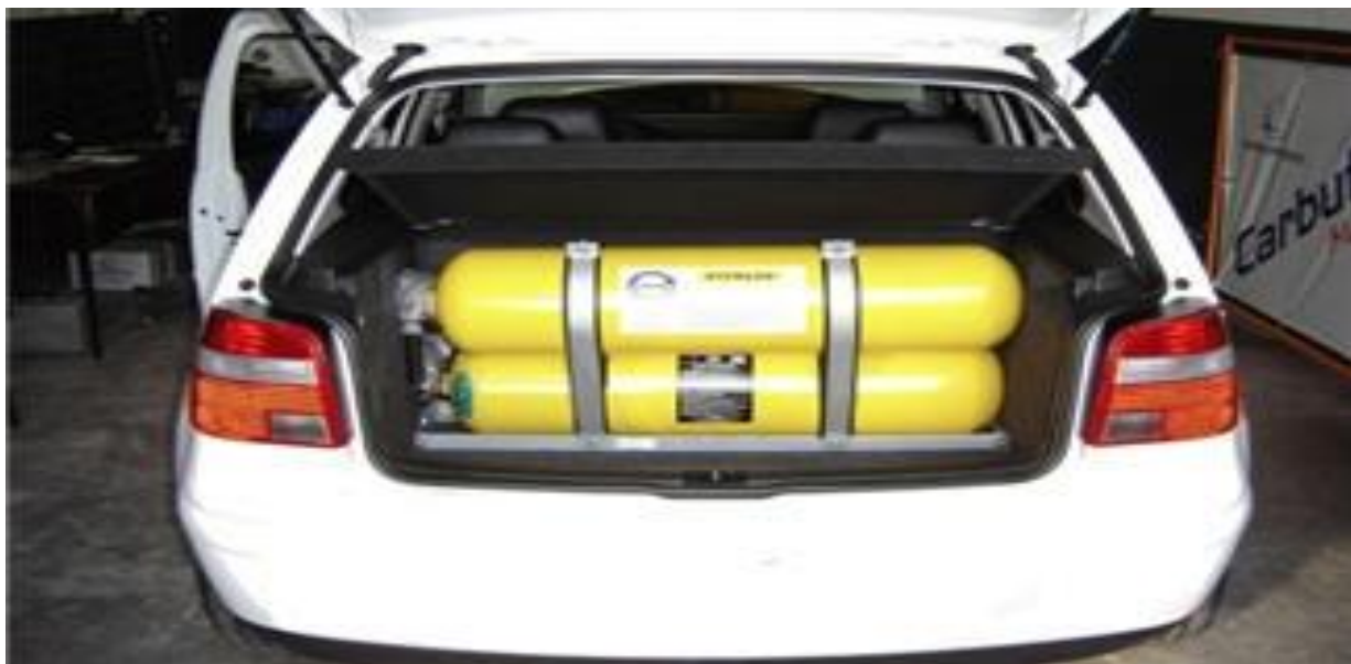
Fig 2.4: Tanks for Storing CNG at Pressure
