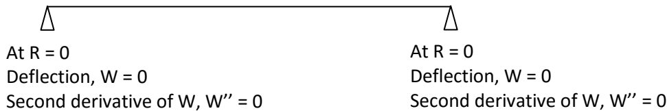
Figure 3.4: SSSS Rectangular Plate's Boundary Conditions.
