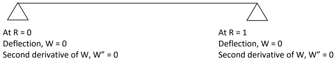
Figure 3.1: SSSS Rectangular Plate's Boundary Conditions.
