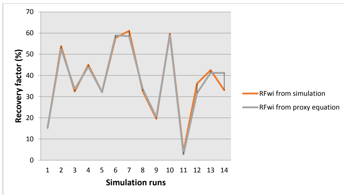
Fig. 4: RF wi Comparison from Simulation and Proxy Equation.
