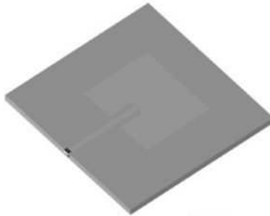
Fig. 2.15: Diagram of Micro Strip Antenna (Elprocus, 2023)
