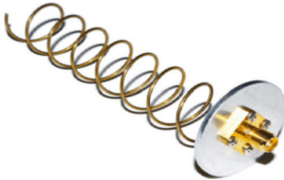
Fig. 2.9: Diagram of Helical Antenna (Elprocus, 2023).
