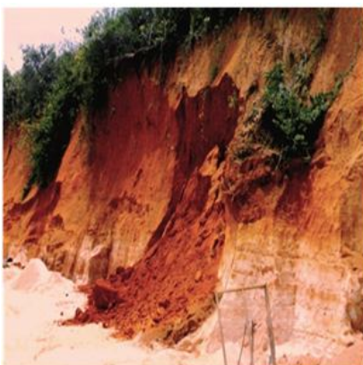
Plate 3a: Abandoned borrow pit showing old slide surface and recent slumping b: Active borrow pit with rapid sliding and palm trees hanging next to pit crest often sliding and causing damages to the excavator c: Heavy duty excavator at work
