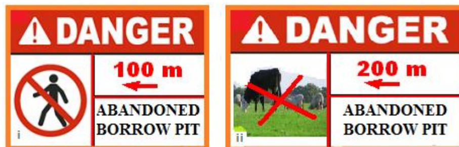
Figure 7b: (i) Danger; Movement Restricted, abandoned borrow pit 100 m ahead (ii) Danger; Grazing Restricted, abandoned borrow pits 200 m ahead
