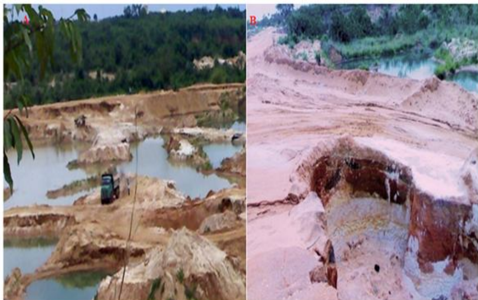
Plate 2a: Selective mining of sand causing dangerous landscape b: Access roads and drive way to the pits is often death traps caused by erosion
