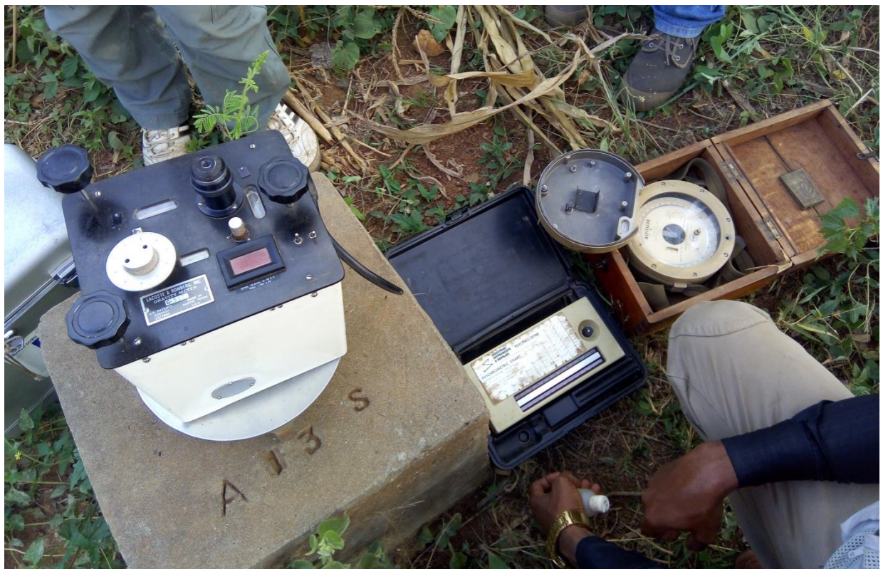
Plate 3.1: Lacoste and Romberg Gravimeter (G512) used for Data Acquisition
