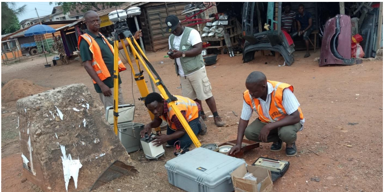
Plate 3.5: Hemisphere DGPS Data Acquisition
