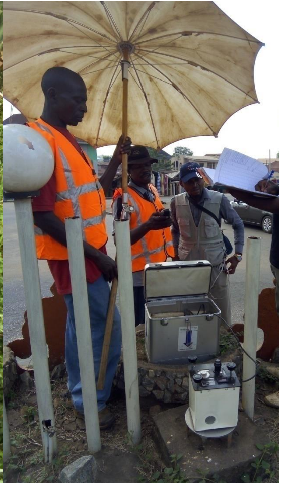
Plate 3.6: Data Acquisition under a protective umbrella to prevent thermal shock
