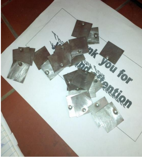
Figure 3.1 : Coupons used for weight loss analysis.
