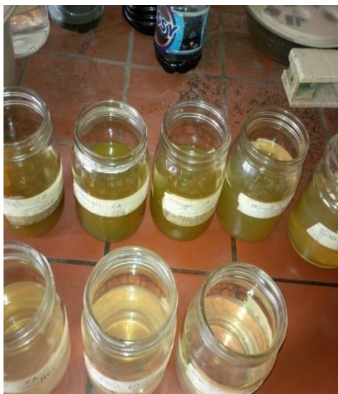
Figure 3.2 Different prepared corrosive environment used for weight loss analysis.
