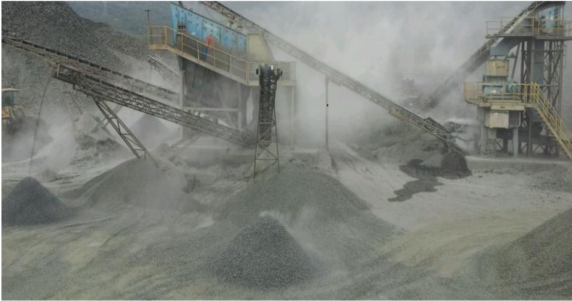
Plate 1: Generation of Particulate matter and Suspended Particulates at the Quarry crushing section Ezizama Quarry (Field School 2014)
