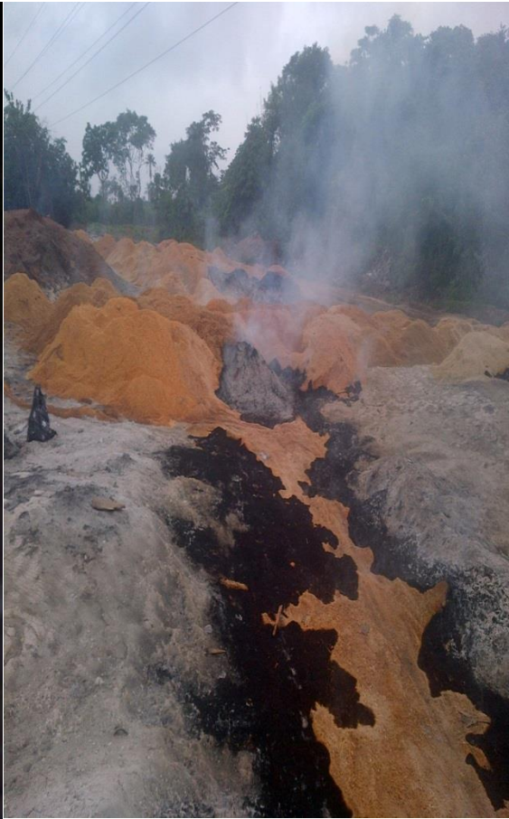
Plate 4: SDA from open air calcination method
