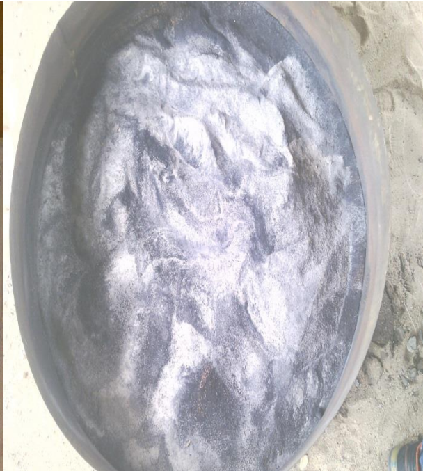
Plate 2: Open-air Calcination of RHA
