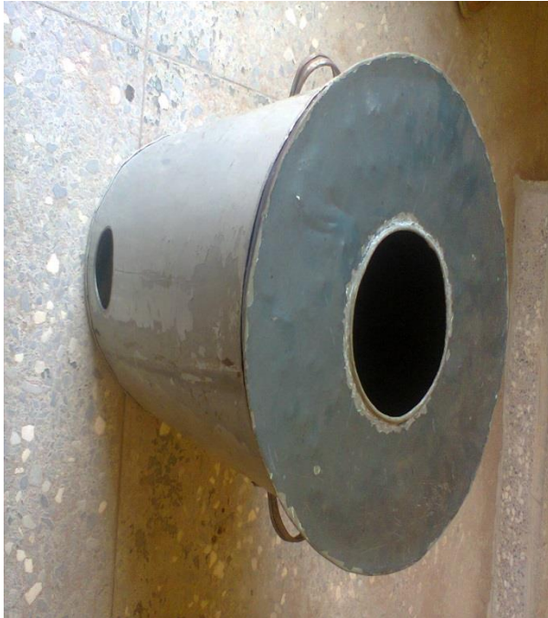
Plate 1: Local stove for burning RHA and SDA
