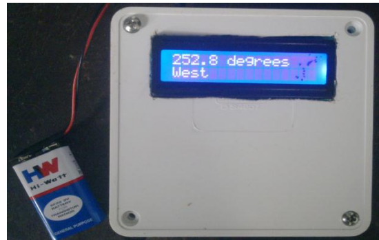
Fig 16: A picture of the completed digital compass
