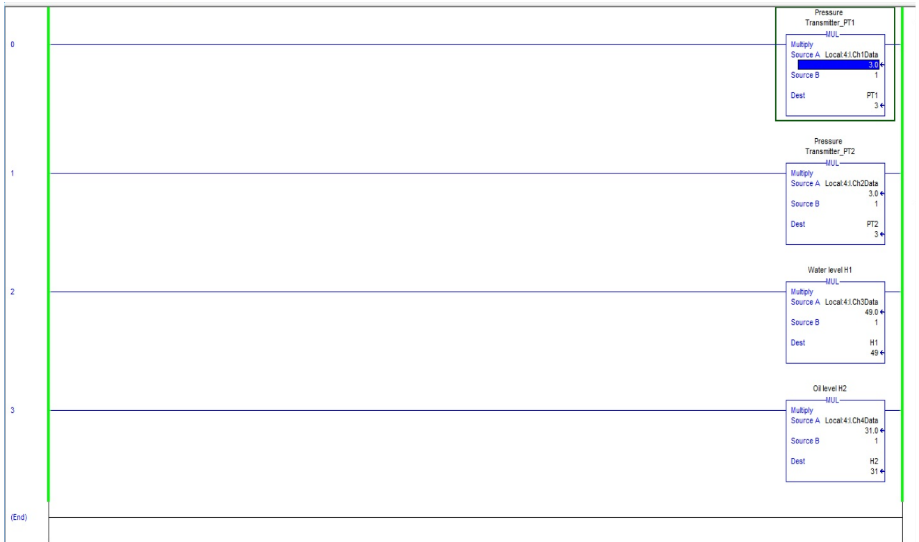
Figure 3.21 PLC Logic for Analog Pressure Low-Low Trip for PT1=3Bar
