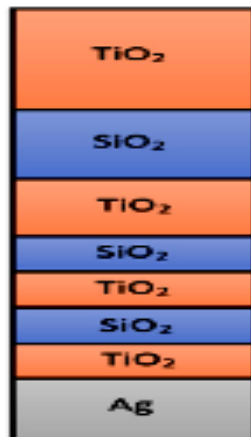
Fig 2.24: Scheme for the implemented structure (Kecebas, et al, 2017)
