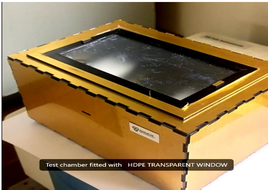
Fig. 3.9: Test chamber before preloading with the selective radiative surfaces
