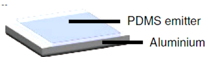
Fig.2.14: Schematic diagram of the planar PDMS/metal thermal emitter (Zhao, et al, 2019)
