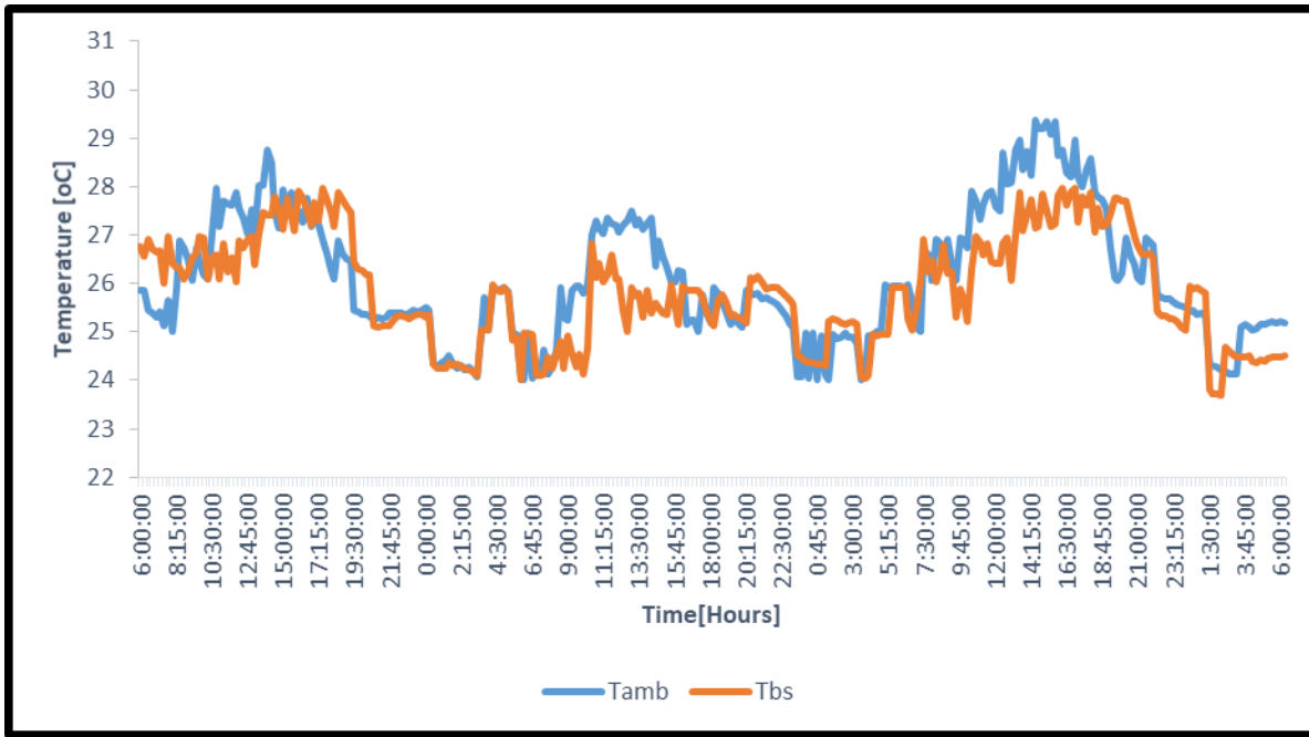
Fig. 4.8: Experimental cooler temperatures of BaSO 4 , and Ambient during August 10-13, 2023 in Afikpo, Nigeria
