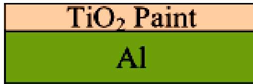
Figure 2.6: Schematic of Coating aluminum substrate with white paint based on \text{TiO}_2 (Harrison and Walton, 1978)
