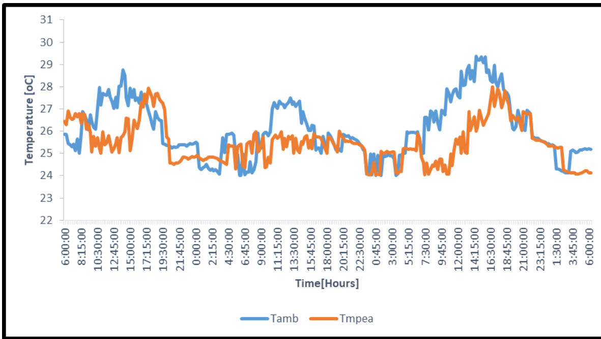
Fig. 4.7: Experimental cooler temperatures of MPEA, and Ambient during August 10-13, 2023 in Afikpo, Nigeria
