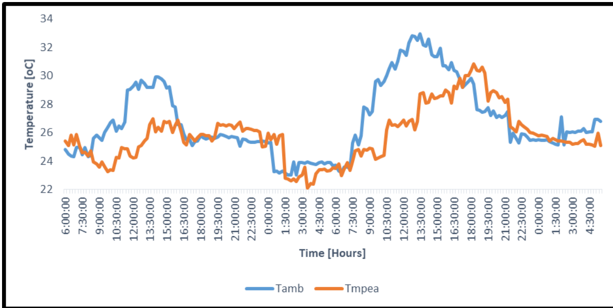
Fig. 4.5: Experimental cooler temperatures of MPEA, and Ambient during July 16-17, 2023 in Afikpo, Nigeria
