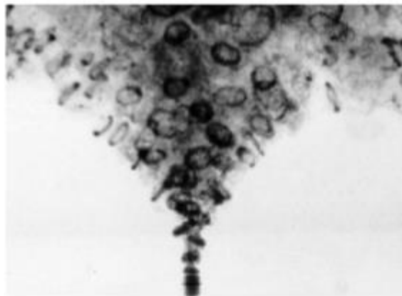
Figure 2.12 Blooming water Jet at Re \approx 20000 (Reynolds, Parekh, Juvet, & Lee, 2003)
