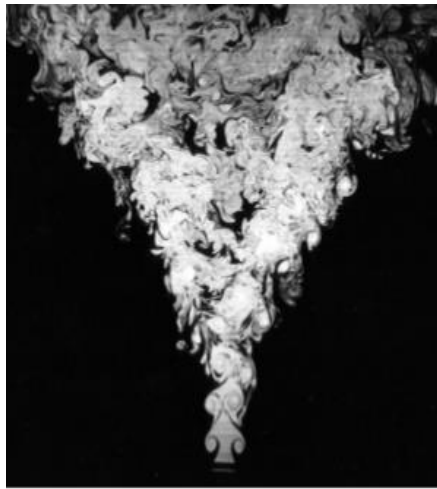
Figure 2.11 Bifurcating water Jet at Re=4300 (Reynolds, Parekh, Juvet, & Lee, 2003)
