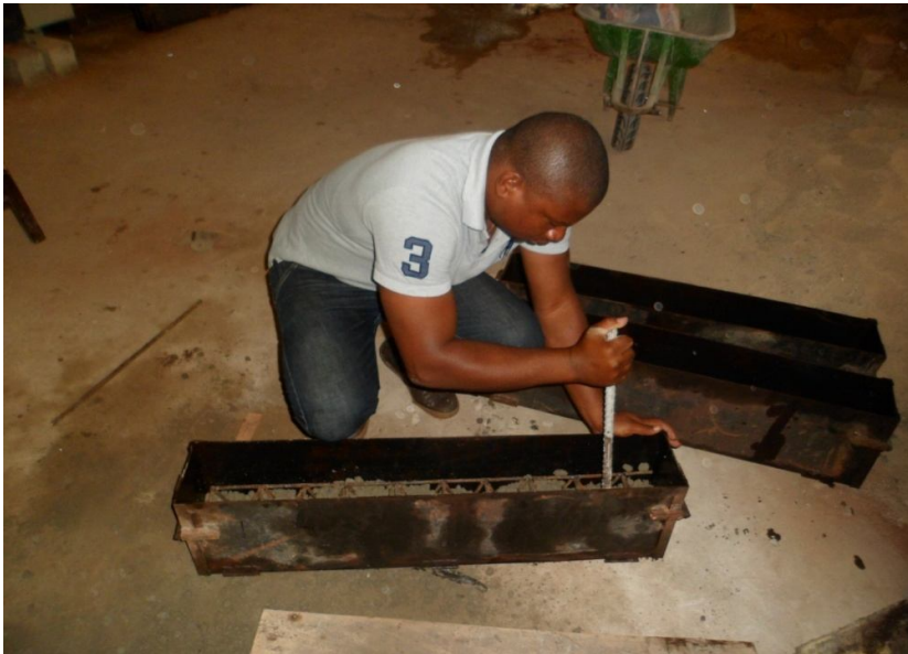
Plate A.9 Ramming of Concrete in beam mould containing truss reinforcement beam
