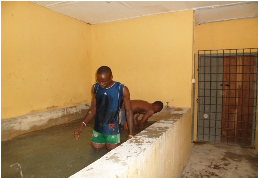
Plate A.12 Curing tank containing beams and cubes
