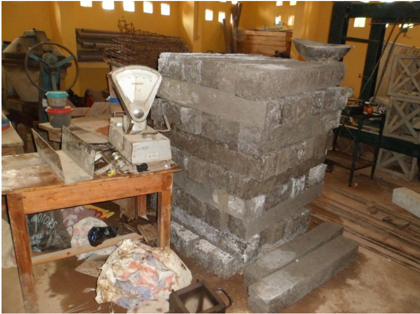
Plate A.13 Beams ready for crushing after curing
