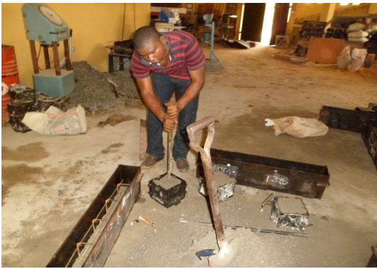
Plate A.9 Ramming of Concrete in beam mould containing truss reinforcement beam
