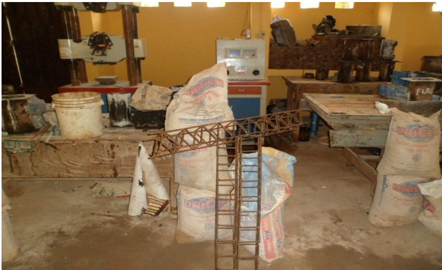
Plate A.1 Fabricated Truss Reinforcement.
