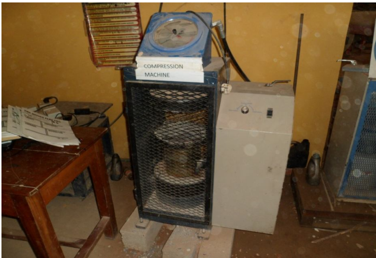
Plate A.16 Concrete compressive Testing Machine
