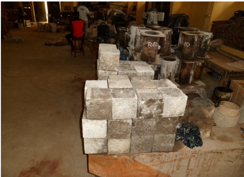
Plate A.14 Cubes ready for crushing after curing
