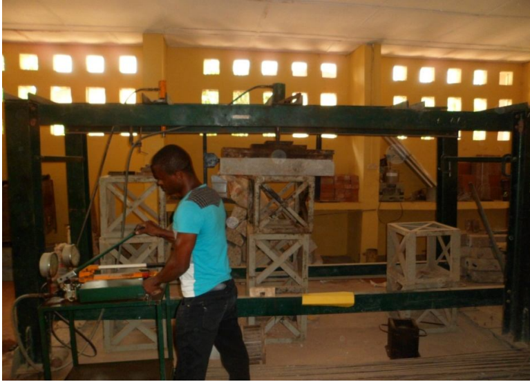
Plate A.15 Crushing of beam in Magnus frame
