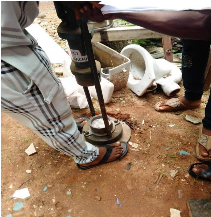
Photo showing the experiment on aggregate impact value test of aggregate for road construction
