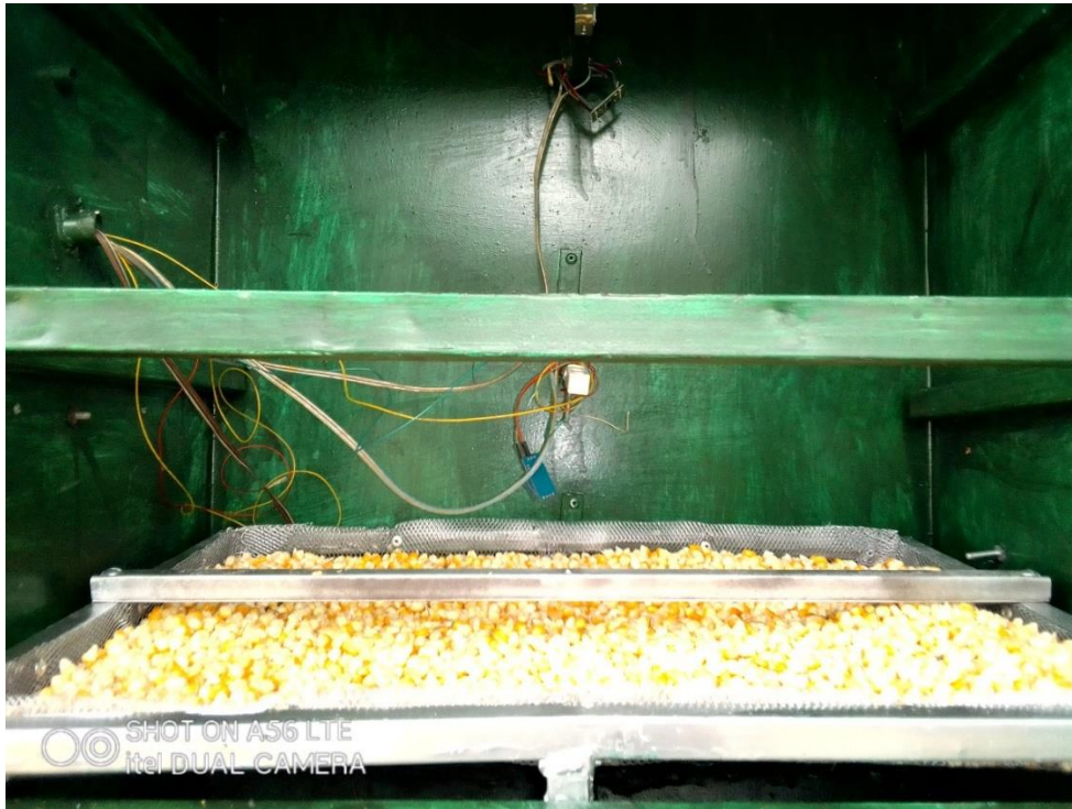
Plate 3.9: Fresh maize grains during drying in the hot air tray dryer
