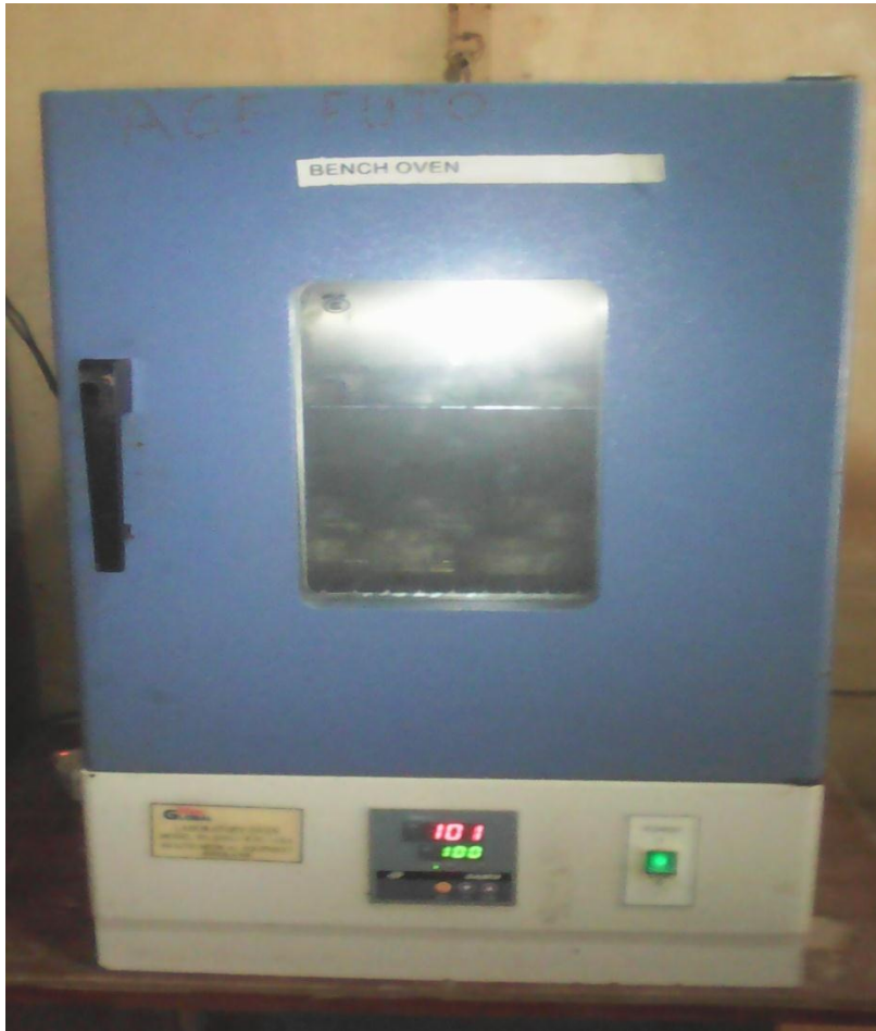
Plate 3.2: A bench laboratory oven (Model DHG – 9101) (range 50 – 300 o c) for the moisture content test
