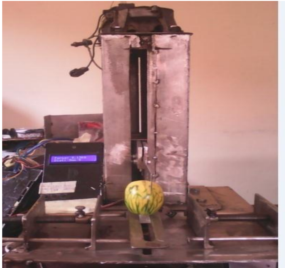
Plate 3.10: Cutting edge just above sample during cutting operation
