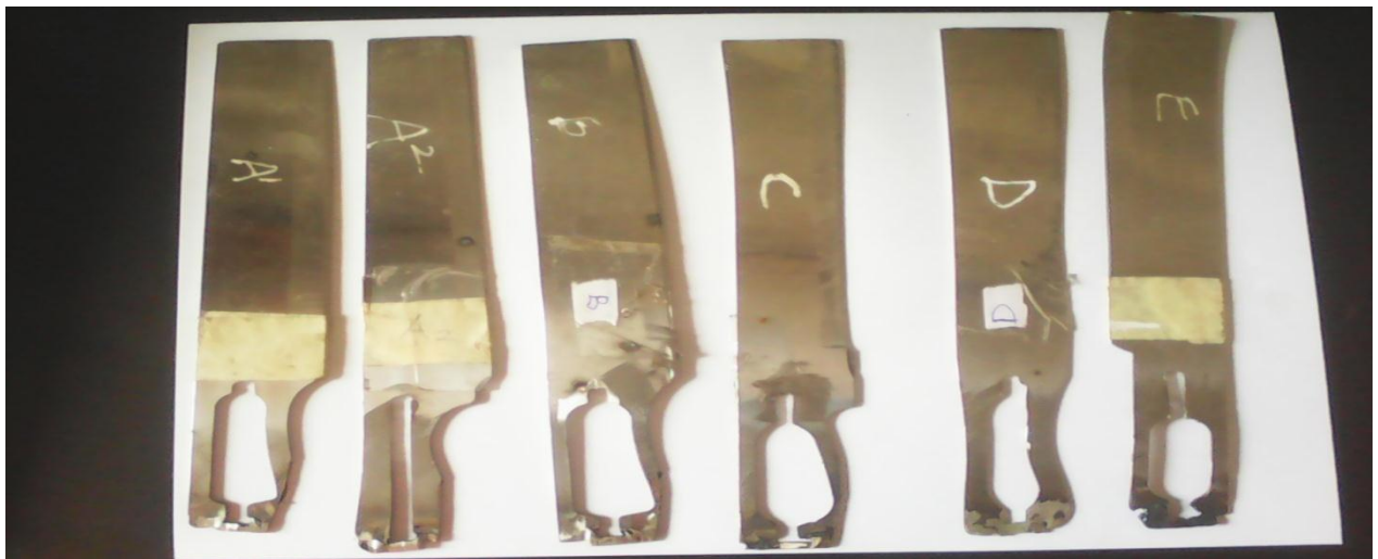
Plate 3.8: Fabricated cutting tools of different edge angles
