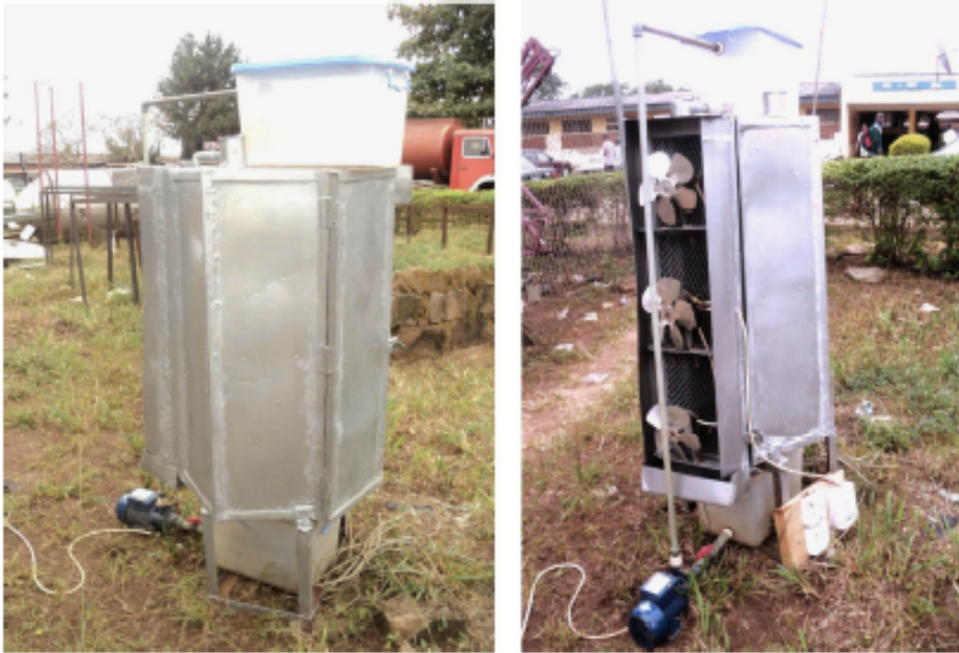
Plate 2.7: Prototype of the Active Evaporative cooling system (Ndukwu et al., 2013)
