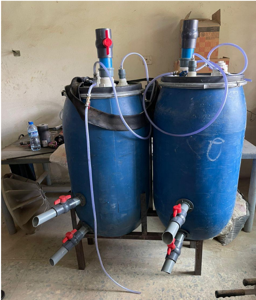
Plate 3.1: Plate showing the constructed mini- digester used for the Biogas production
