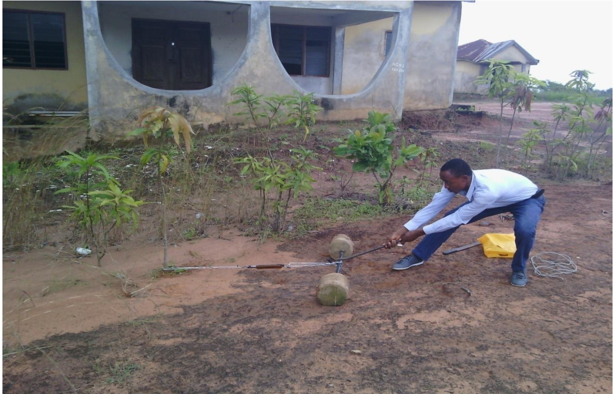
Plate 3.1- Lateral uprooting test in Nguzu-Edda Erosion Site 1
