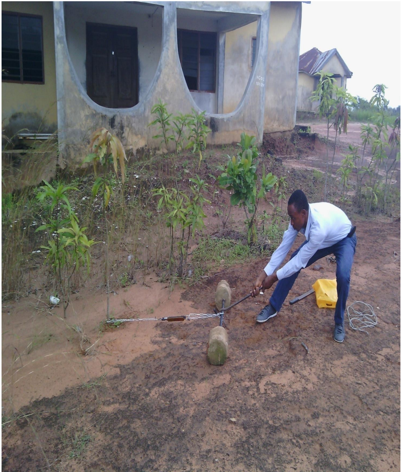
Plate B4 - Lateral Uprooting Test at Nguzu Edda Erosion Site 2
