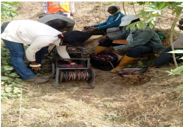
Fig. 3.5: Field Layout of Schlumberger Array
