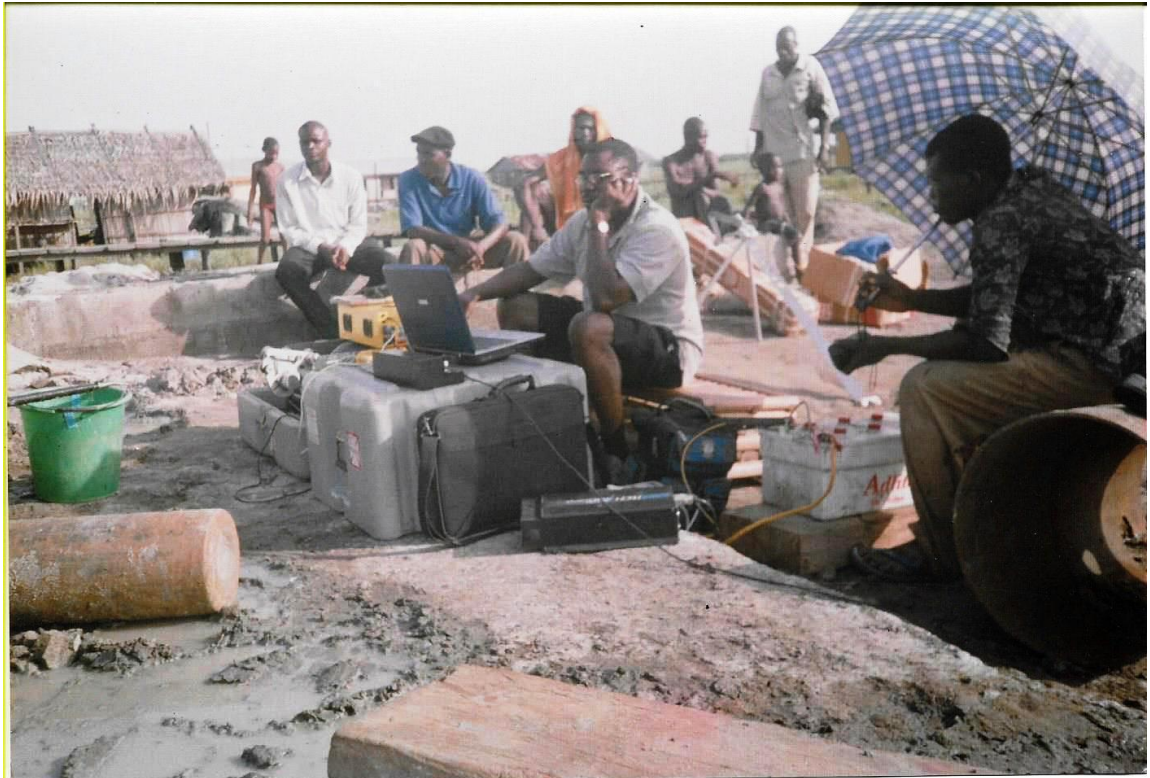
Figure 3.5: Mount Sopris MGX 11 Logging Equipment
