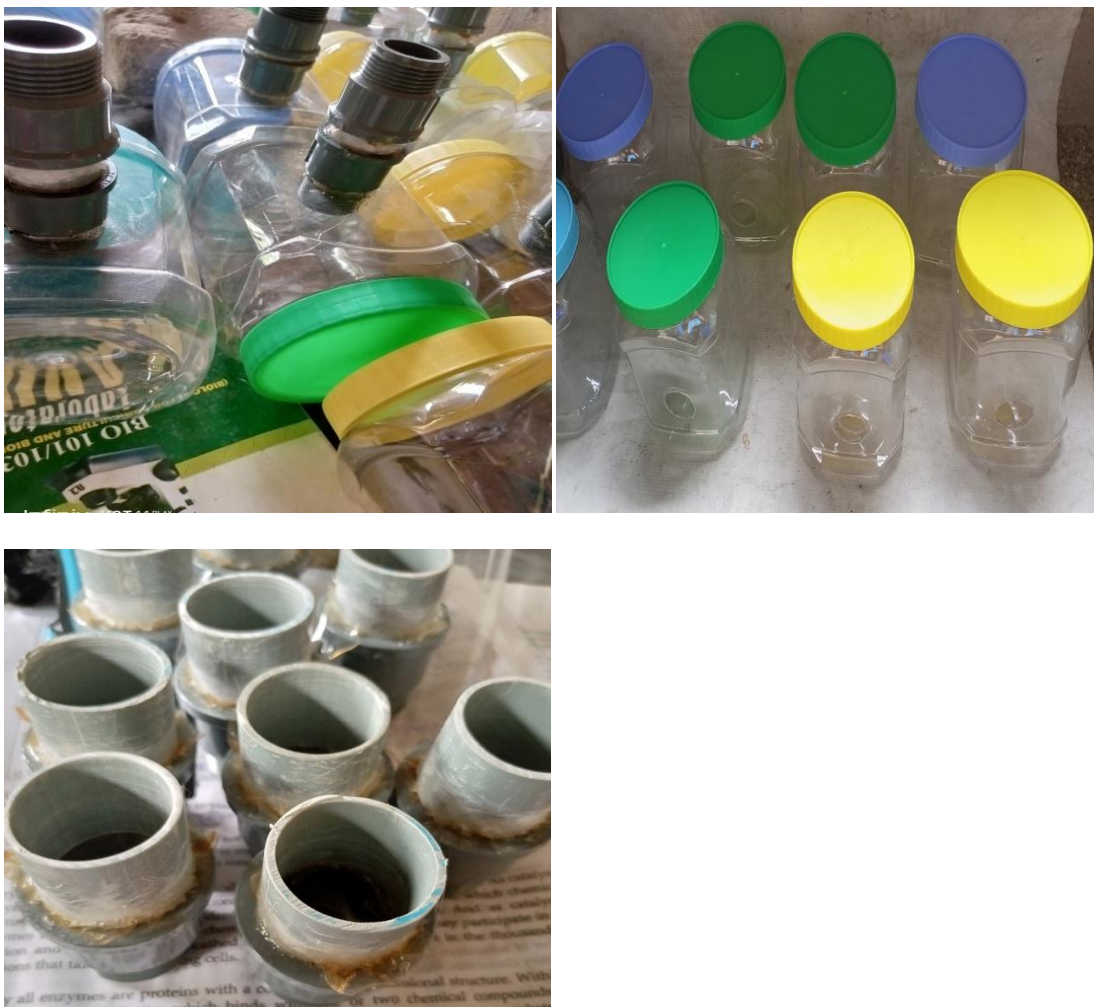
Plate 3.2: Plastic materials used in the construction of the MFCS
