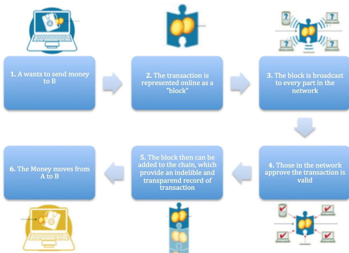
Figure 2.1: A Simple Example of how the Blockchain technology works with a transaction of money (Crosby et al., 2016).
