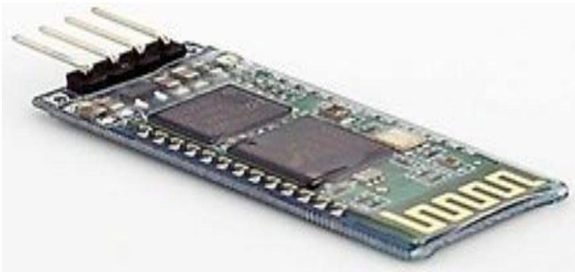
Figure 2.1: HC-05 Bluetooth Module (source Bhavik et al., 2016)
